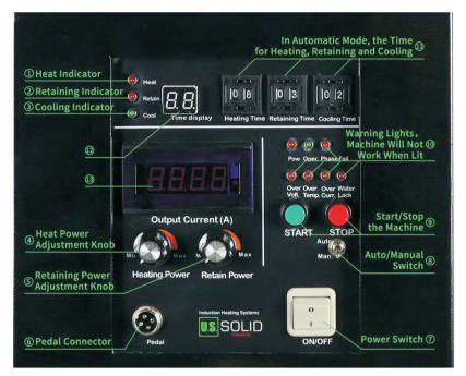
① Time (in seconds) given between zero and 99 seconds. Can be increased using the button **below** the numbers and decreased using the button **above** the numbers.
