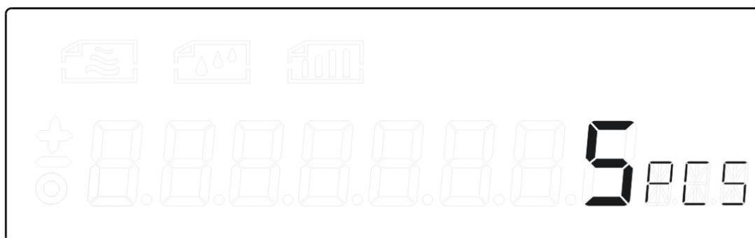
5. After the test is finished, press “ON” to select “weight”, and press “O/T” to confirm to exit and return to the weighing interface.
