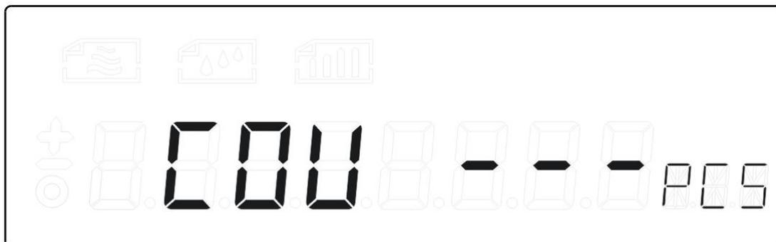
4. The operation can be started when the “COU ---” disappears and the corresponding number appears.
