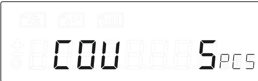
3. Press “ON” to select the quantity and put the corresponding quantity of samples. Press “O/T” to confirm and “COU ---PCS” will be displayed.
