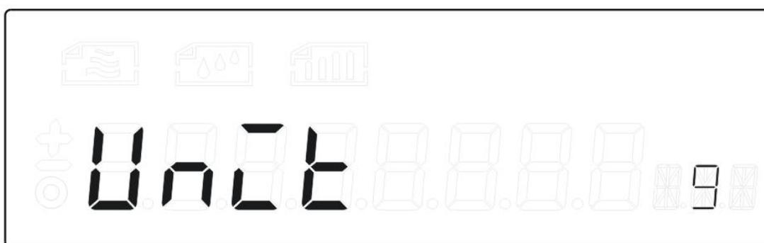
3. Press “ON” to select required unit and confirm by pressing “O/T”.
